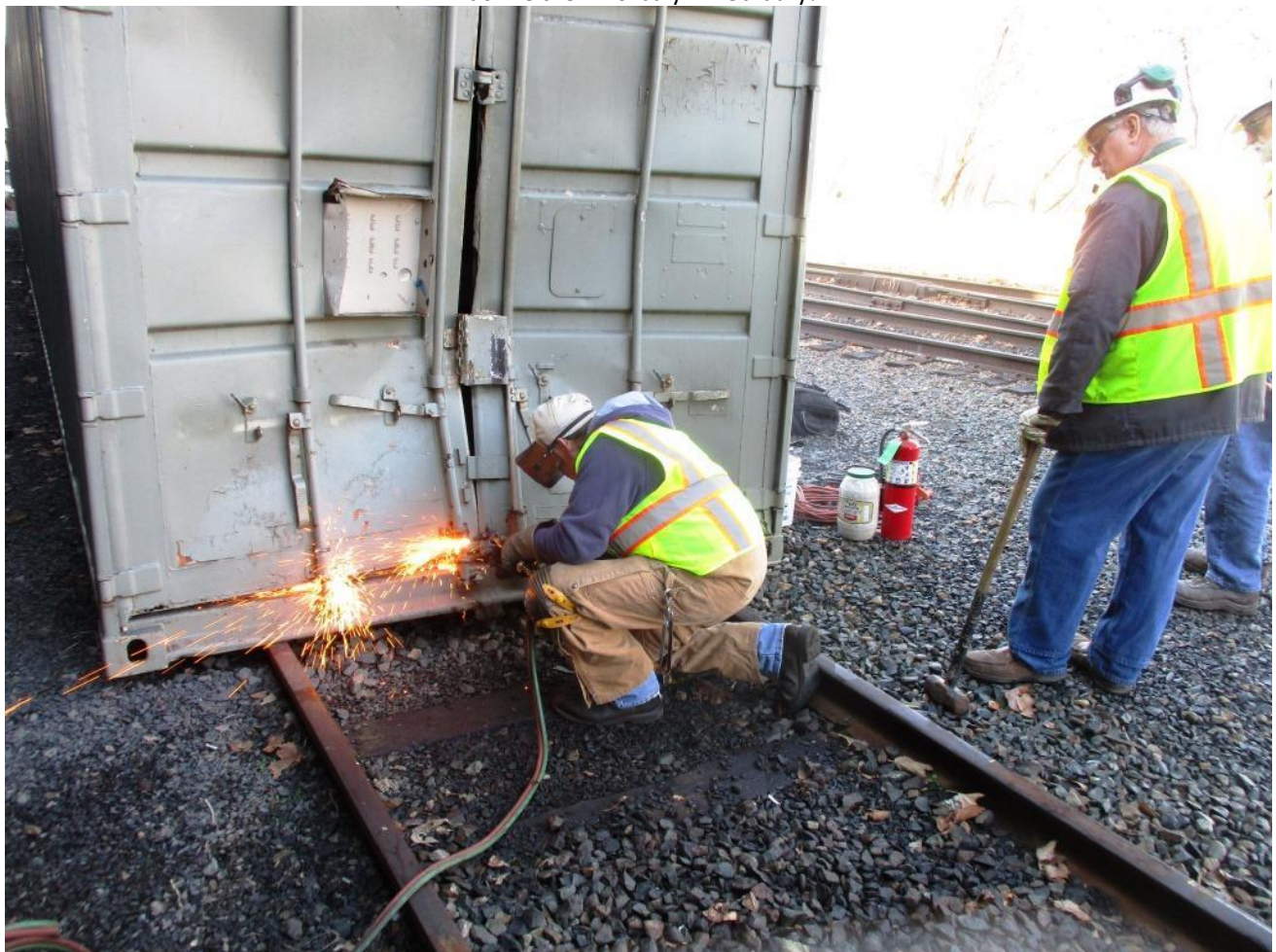
Cliff cuts through the bottoms of the locking rods
